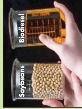
Biodiesel is an environmentally friendly fuel, burning much cleaner than fuels made from oil. In Minnesota, most biodiesel fuel is made from soybeans, which are high in oil. Like ethanol, it is renewable because it comes from crops that can be grown every year.
