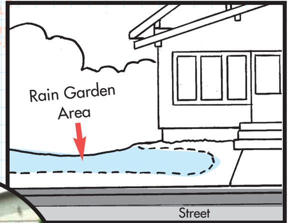
Rain gardens are gardens designed with a dip in the center to collect rain and snow melt. When planted next to hard surfaces such as sidewalks and parking lots, rain gardens collect runoff water. This water is filtered as it seeps slowly into the ground. Rain gardens help keep runoff out of storm sewers, or from running directly into our lakes and streams.
