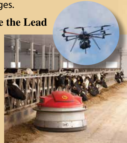
A drone surveys fields and a robot pushes feed so cows can reach it.
